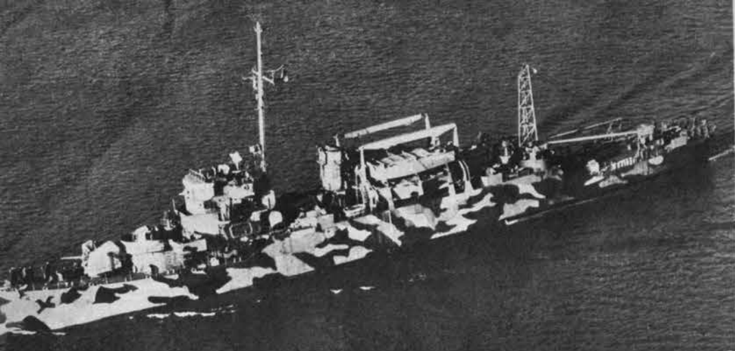
High-speed transport is the Navy's fastest assault troop carrier. A destroyer escort conversion, the trim APD is identified as such primarily by the landing craft it carries amidships.
